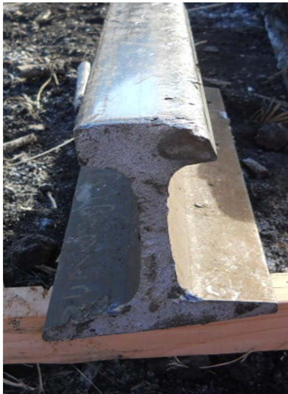
Two separate detail fracture defect were recovered in the wreck. One 25% and one 20%. Rail was scheduled to be replaced 2015.
