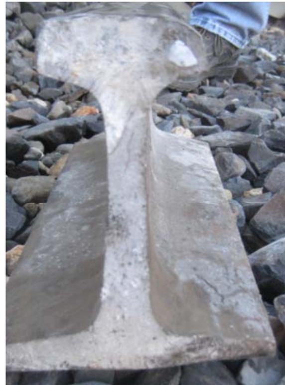
Two separate detail fracture defect were recovered in the wreck. One 25% and one 10%. Rail was scheduled to be replaced 2015.
