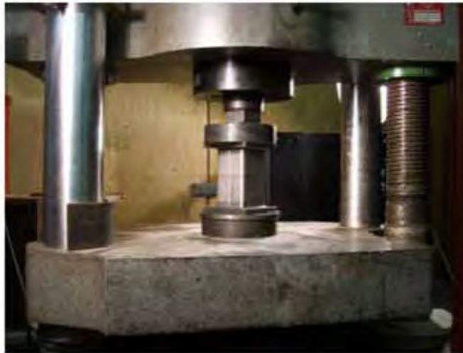
Figure 83. Example of a Quasi-static Test of a CEM Component
