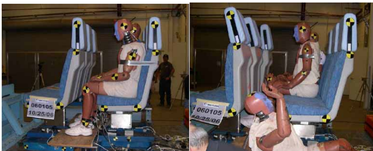
Figure 13. Pre- and Post-test Photos of Forward-Facing 8g Sled Test
