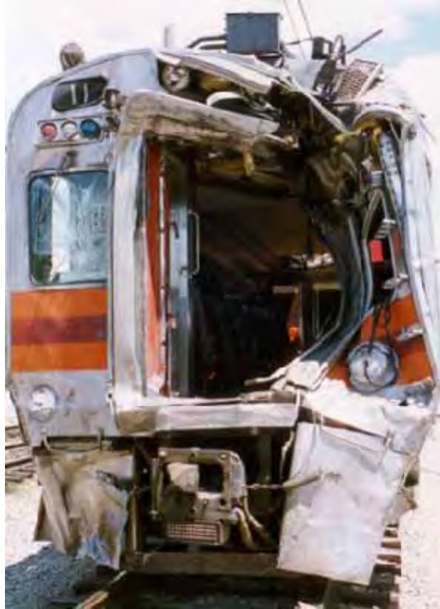
Figure 34. Lead Cab Car after Striking Truck at Highway-rail Grade Crossing (Portage, IN - 1998)
