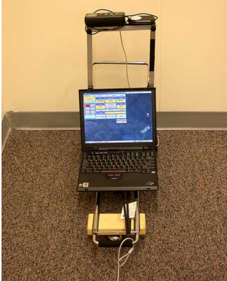
Figure C2. Apparatus for measuring average illuminance levels: Consists of a hand-held illuminance meter with sensor, an analog-to-digital converter (if not built into the meter), a notebook computer, a luggage cart with an added bracket to hold the sensor, an extra caster, and a towline.
