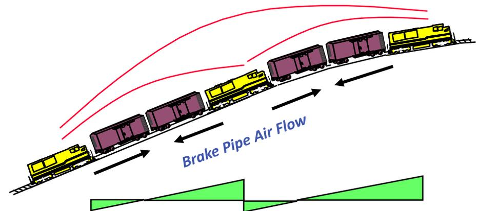
Draw Bar Forces reduced when locomotive power and braking is distributed throughout the train
